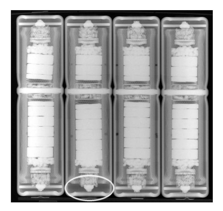
The image above is a neutron radiograph of four air bag initiators. The second part from the left is missing an o-ring at the bottom and is therefore dysfunctional. Due to the ability of neutron radiography to image rubber and other hydrogenous materials so well, it is an effective complex component reliability testing technique
