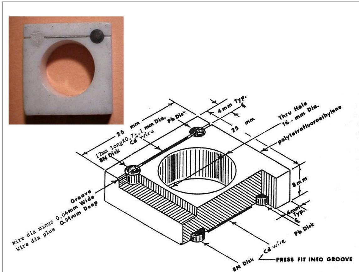
**Figure 17.1: Picture and drawing of Beam Purity Indicator**
