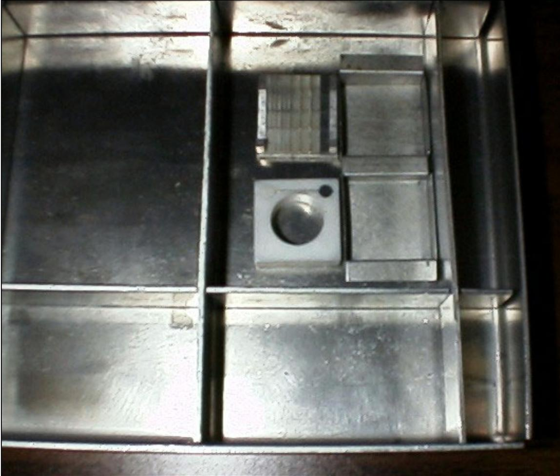
**Figure 17.4: Correct placement of Indicators in part holder**
