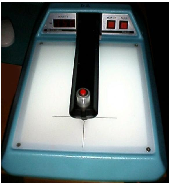
**Figure 17.7: Light transmission densitometer**
