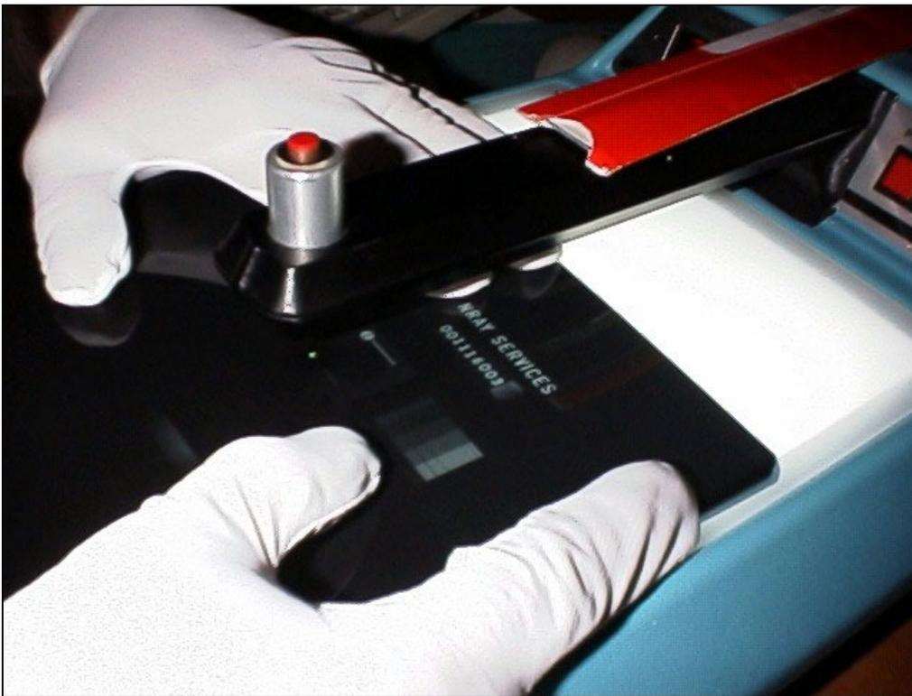
**Figure 17.9: Measuring density of boron disk with densitometer**
