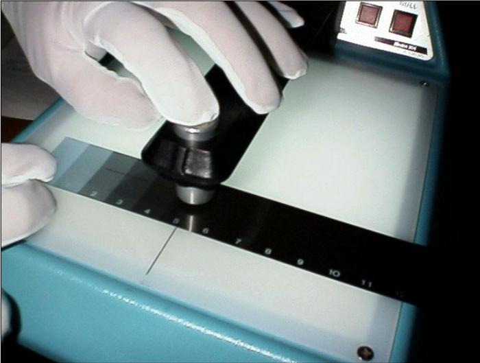
The densitometer should be calibrated before use with a step-wedge calibrated to a national standard.
