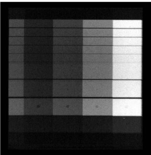
The SI consists of a step wedge containing gaps and holes of known dimensions. Visual inspection of the image of the SI provides subjective information regarding total radiographic sensitivity with respect to the step-block material as well as subjective data regarding detrimental levels of gamma exposure.
