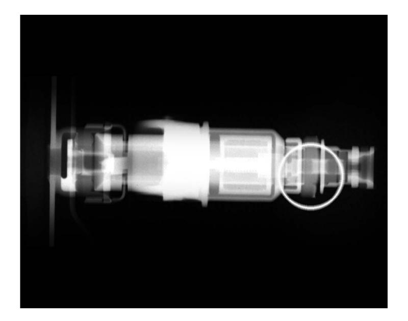
The image above is a neutron radiograph of a fuel injector base component. The o-ring between the injector and the base is identified in the image by a circle. It is clearly seen that the o-ring in question is misaligned. Neutron radiography is a very useful and effective technique for identifying missing or misplaced o-rings.
